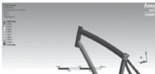
Figure 9. Von Mises stress distribution between the head and top tube
