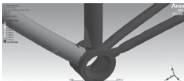
Figure 8. Von Mises stress distribution between the seat and down tube
