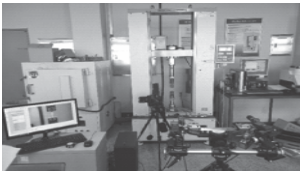
Figure 3. Two typical DIC techniques and their imaging models and system.
