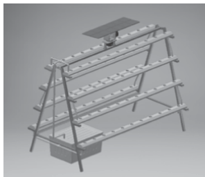
Fig. 2. 3D model of hydroponic vegetable growing using solar energy in Autodesk Inventor software.
