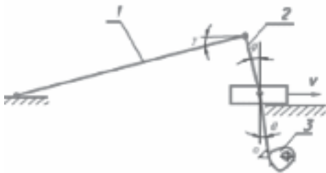
Figure 4. Diagram of acceleration mechanism 1- Eject bullets pice; 2- Accelerometer pice; 3-Surface.
